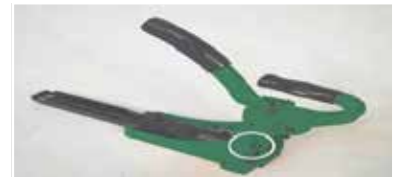
Mechanism for adjusting the depth of staple penetration
